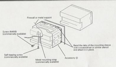
Make sure that the unit is installed securely in place. If the unit is unstable, it may malfunction (eg, the sound may skip).
